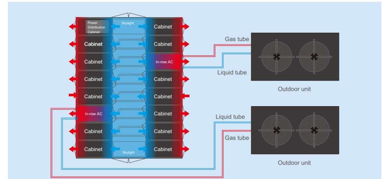
When the outdoor unit is higher than the indoor unit: the vertical height difference between indoor and outdoor units should not exceed 20m; when the indoor unit is higher than the outdoor unit: the vertical height difference between indoor and outdoor units should not exceed 5m.
