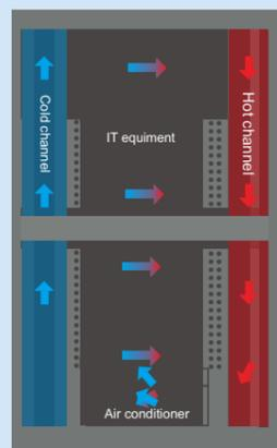
Note: The layout can be adjusted according to the equipment layout.
